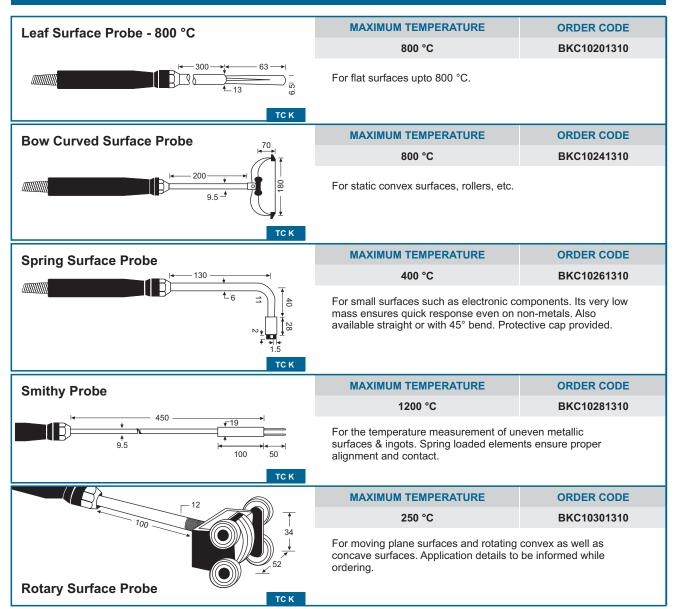
TC K (thermocouple) handle probes are supplied with a 1 metre coiled green PVC cable.
