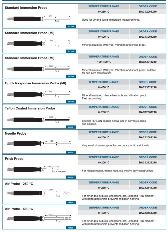
RTD handle probes are supplied with a 1 metre PVC cable.
